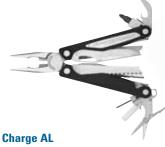
The Charge AL handles with hard anodized aluminum scales have rounded edges for grip comfort. It includes needle-nose pliers, wire stripper, bottle/can opener, saw, serrated knife, fixed lanyard ring, wire cutters, scissors, bit drivers, eight double-ended bits, removable pocket clip, a quick-release lanyard ring, a diamond-coated file and a 154CM clip-point knife. A sheath is included.
