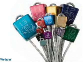
Wedgies are built with a double taper to fit slight flares and more typical cracks alike. Available individually or in sets, each is extruded and machined from 6000-series, aircraft-quality aluminum alloy and anodized for instant identification on your rack. Slung with strong, braided steel cable, they're built for years of use.
