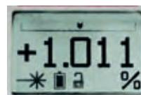
**Large clear display** with easy to read grade numbers, line indication, battery status, and level indication.
