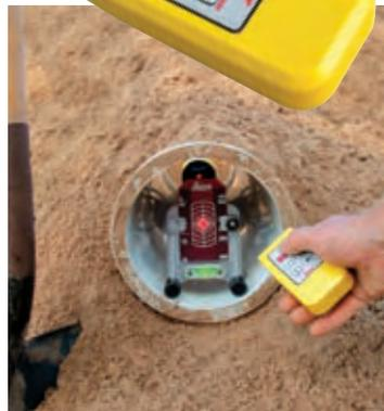
**Multi-function remote** works up to 150 m (500 ft) for line control and other features.
