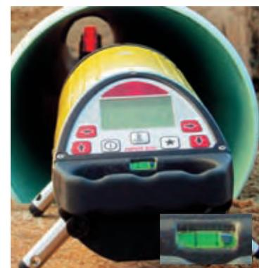
**Automatic grade compensation** with the housing rolled up to  $\pm 3^\circ$ , the Piper will compensate and correct for the grade errors.
