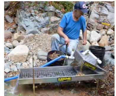
Model 176124CA Concentrator 12 inches wide x 7 feet long
