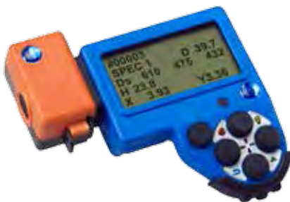
Image shows DP Postex module on DP II terminal
