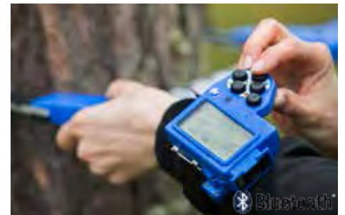
The DP II Computer terminal as a stand-alone unit can be used for example when collecting and registering biotopes on plots. Work with designated software application and DP GPS add-on to register plot coordinates and other data.
